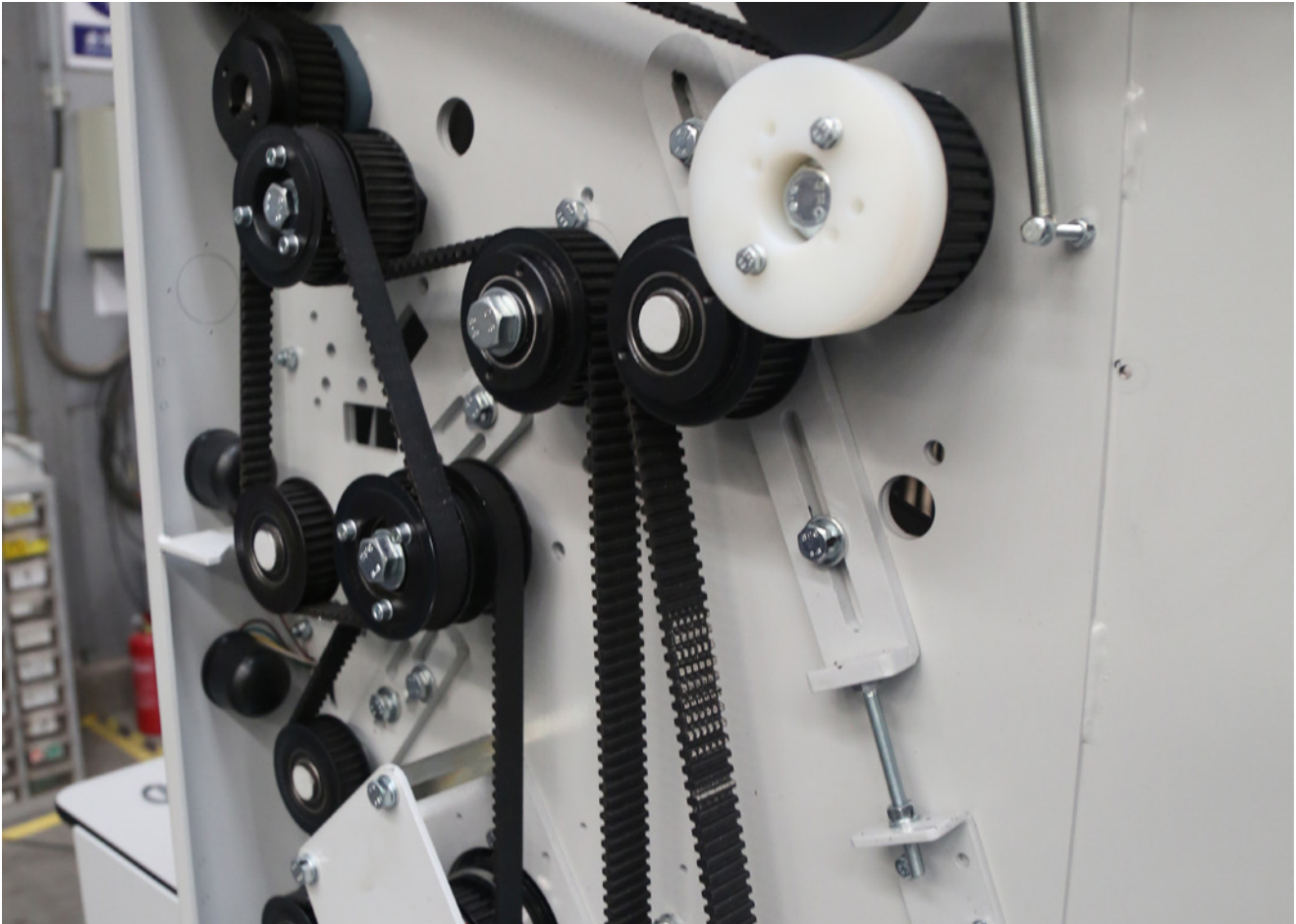
Toothed belt drives in the lateral fold section for high precision at high operating speeds
