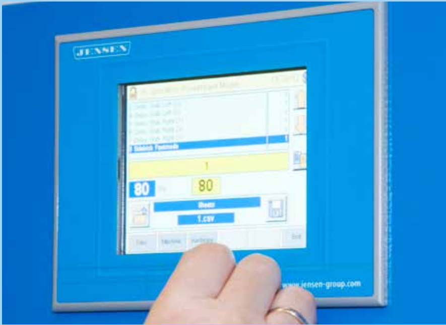
Jentrol HMI PLC and control system with touch-screen
