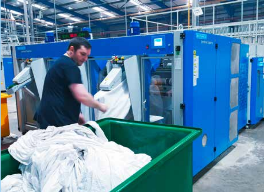
The new 3-station Jenfeed Express Trio is capable of feeding up to 1800 single hospital sheets per hour.
