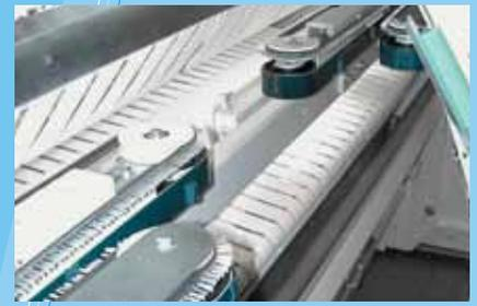
Unique spreading system with double spreading belts and brushes
